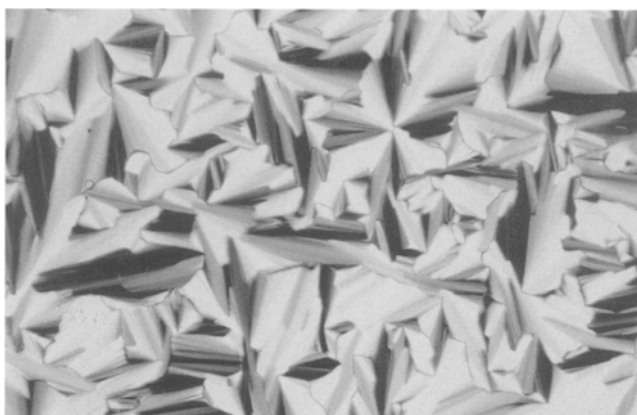
Fig. 7 Fan texture of the partially polymerised \omega -UTAB hexagonal phase (crossed polarising filters, magnification 240). The cylinders lie parallel to the glass slide and the brushes correspond to line disclinations of strength s = +1/2 , where the splaying out indicates variations in the curvature of groups of cylinders about the line disclination. The brushes lie at an angle of 5^\circ to 10^\circ to the polariser and analyser. Edge dislocations between individual fans are indicated by sharp dark lines, (67.7 wt% \omega -UTAB sample at 25^\circ\text{C} )
